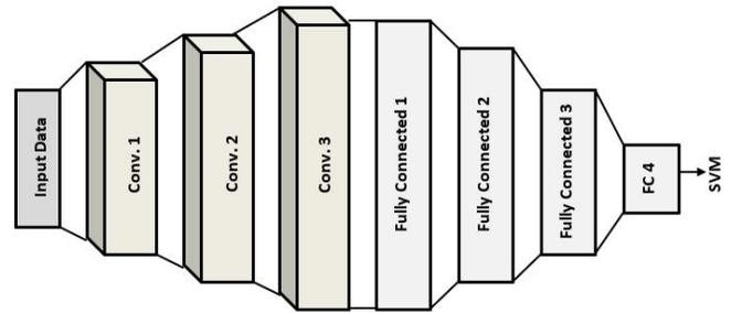
Fig. 2. Proposed network architecture combining convolutional (Conv.) and fully connected (FC) layers.
