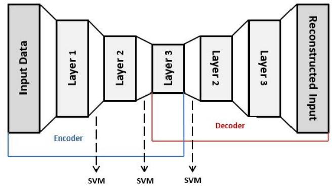
Fig. 1. Architecture of a Stacked Autoencoder for feature extraction combined with SVM for classification.
