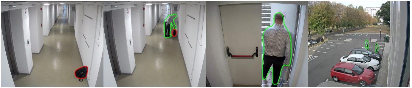
Fig. 2. From left to right: abandoned object that triggered an alarm, detected suspect leaving the baggage, suspect leaving the building, suspect interacting with another person. The person in the third image is 210 \times 500 pixels in dimension, whereas in the fourth image it is of 30 \times 60 pixels.
